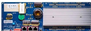
ES485 Communication between battery and inverter Bit rate: 9600bps. ES485 Interface Communication between parallel packs or BMS and PC Bit rate: 9600bps.
